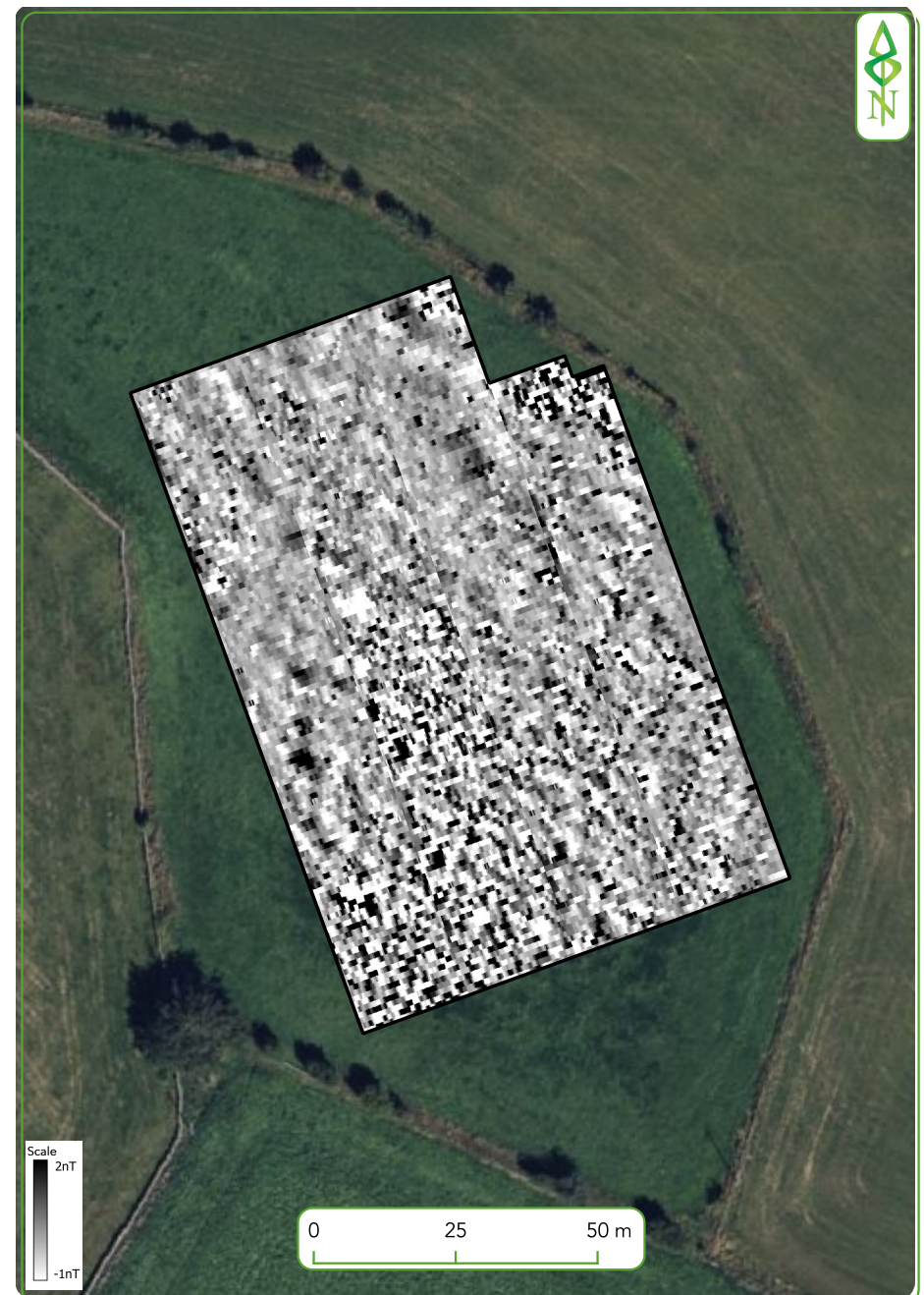
Figure 3. Raw unprocessed gradiometer survey data and minimally processed gradiometer survey data - greyscale plot
