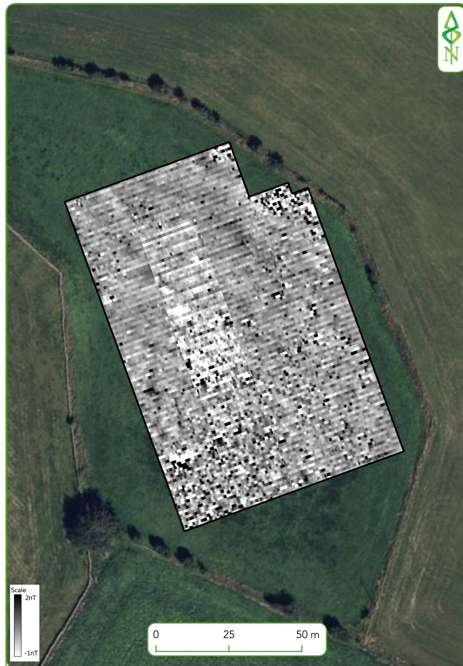
Figure 3. Raw unprocessed gradiometer survey data and minimally processed gradiometer survey data - greyscale plot
